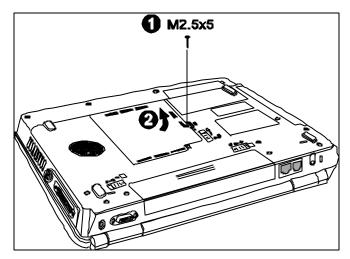
*Figure 4-12 Removing the memory module cover*
