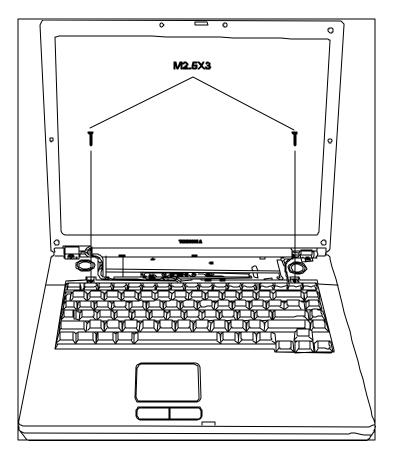
*Figure 4-17 Removing the keyboard*
