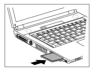
*Figure 4-3 Installing a PC Card*
