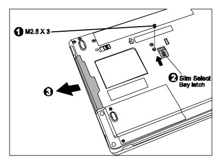
*Figure 4-8 Removing the optical drive module*
