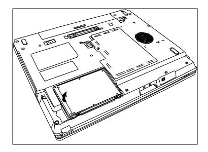
*Figure 4-6 Removing the HDD module*
