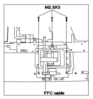
Figure 4-27 Removing the Touch Pad board
