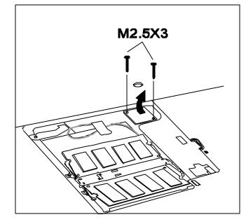
Figure 4-20 Removing the modem module
