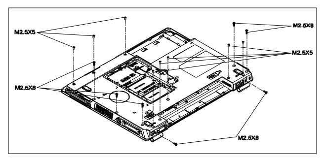
Figure 4-23 Removing screws of the bottom
