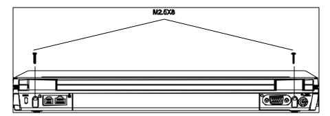
Figure 4-21 Removing the display assembly screws
