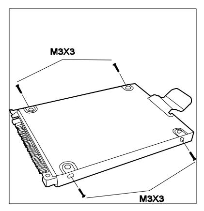
*Figure 4-7 Removing the HDD bracket*
