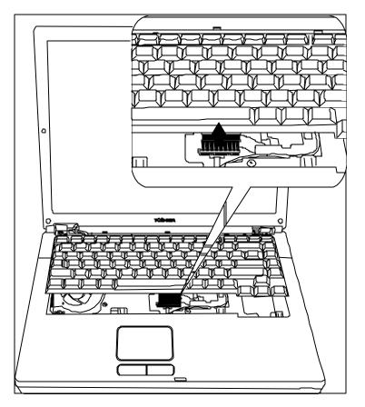
*Figure 4-18 Disconnecting the keyboard cable*
