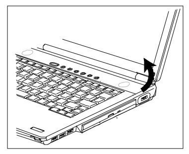
Figure 4-16 Removing the strip cover
