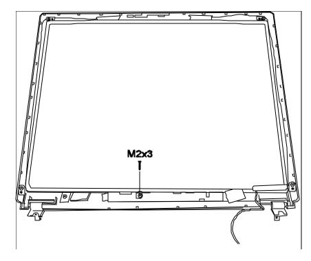
Figure 4-39 Removing the FL inverter board
