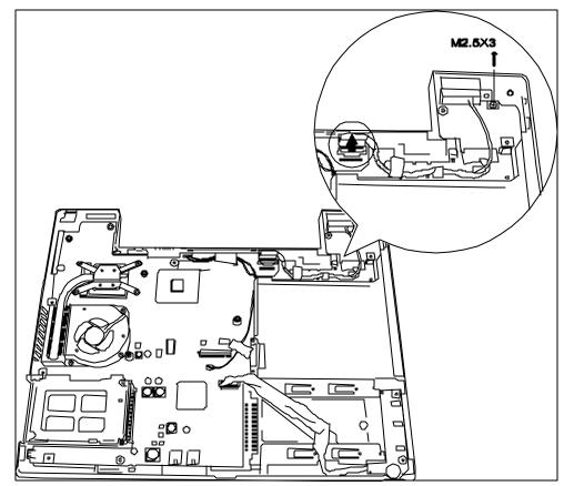
Figure 4-29 Removing LAN board
