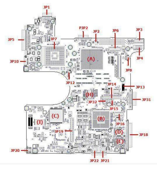
Figure B-1 System board (FRDSY\*) layout (Top)
