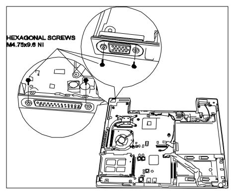
Figure 4-31 Removing the system board
