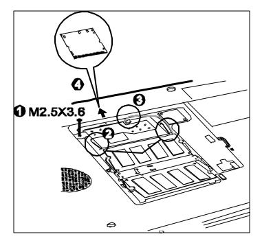
Figure 4-11 Removing the wireless LAN unit
