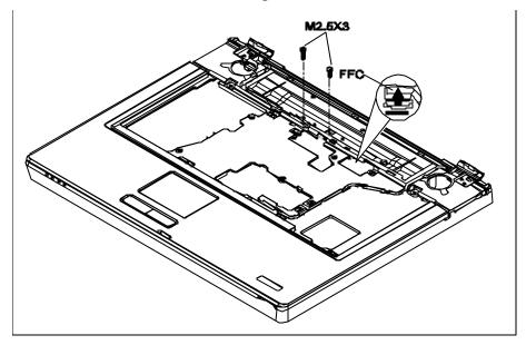
Figure 4-32 Removing the Direct Play Button board
