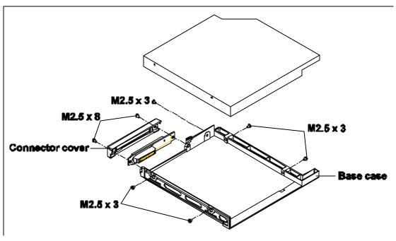
*Figure 4-9 Removing the optical drive bracket*
