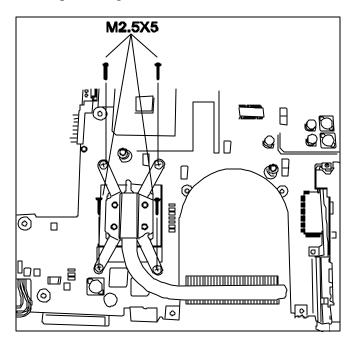
*Figure 4-34 Removing the heat sink*
