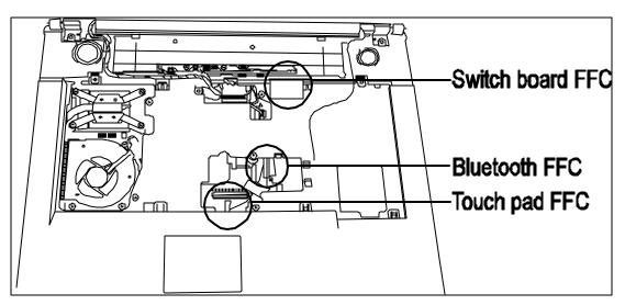
Figure 4-25 Removing FFC cables
