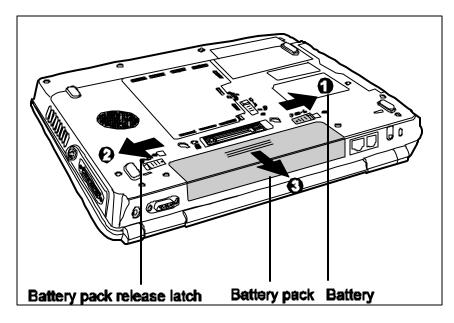
*Figure 4-1 Removing the battery pack*
