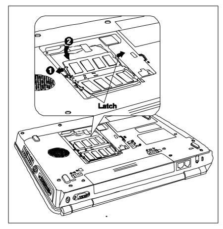
*Figure 4-13 Removing a memory module*
