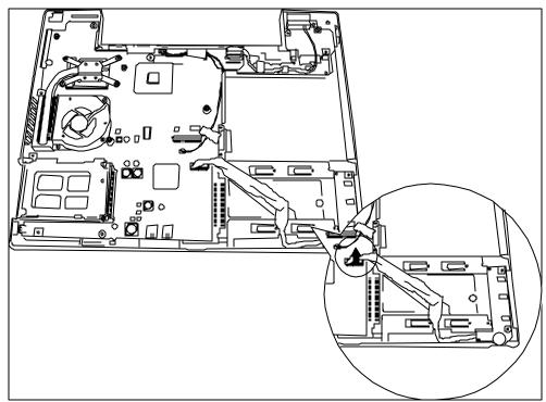
Figure 4-30 Removing USB board
