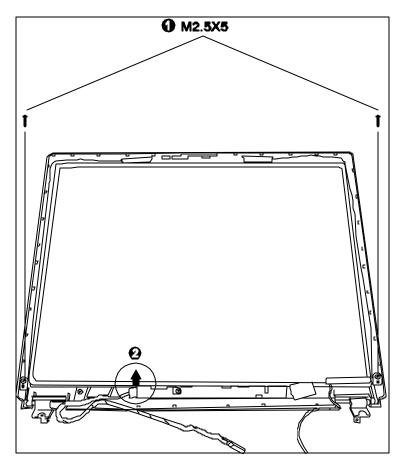
Figure 4-37 Removing the LCD module-1
