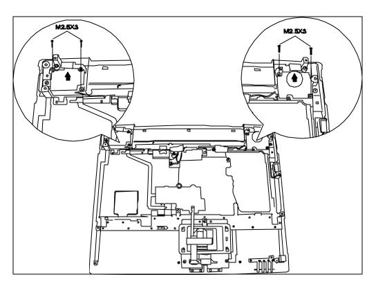
Figure 4-28 Removing the speakers
