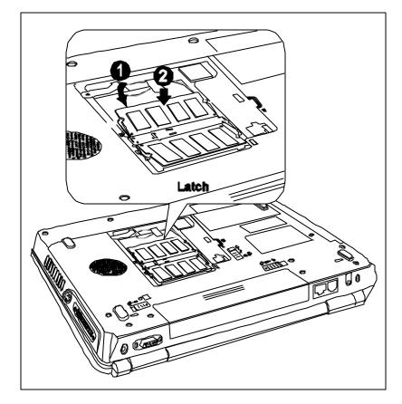
Figure 4-15 Installing an expansion memory
