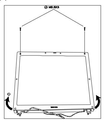
Figure 4-36 Removing the display mask
