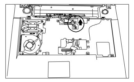
Figure 4-26 Removing Speaker cables
