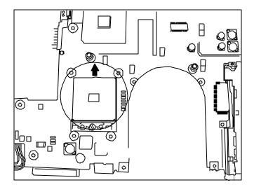
Figure 4-35 Removing the CPU
