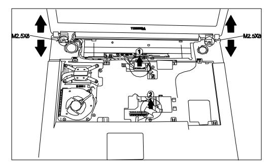
Figure 4-22 Removing the wireless and LCD cables
