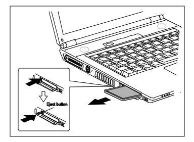
Figure 4-2 Removing a PC Card
