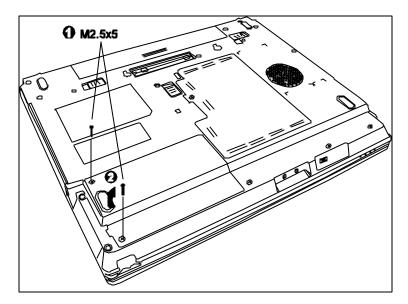
*Figure 4-5 Removing the HDD door*
