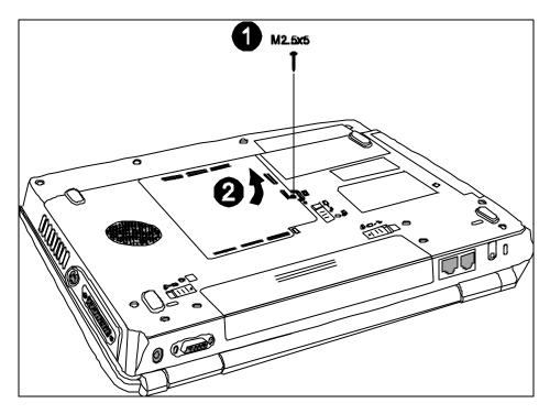
Figure 4-10 Removing the wireless LAN cover
