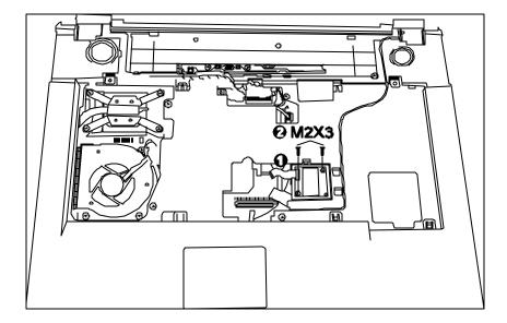
Figure 4-19 Removing the Bluetooth
