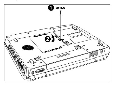
Figure 4-14 Removing an expansion memory cover
